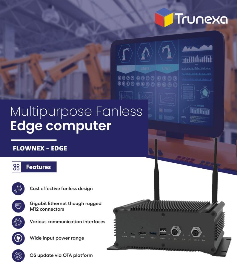
Flownex-Edge is a fanless embedded computer for various industrial applications that demands anti-vibration and anti-shock protection. Flownex-Edge is based on Arm® Cortex®-A53 quad core processor, which operates at speed of 1.3GHz. It offers advanced audio, voice, and video functionality with low power consumption.
